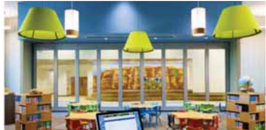
Floor area increased by opening an acoustical glass wall partition with manual and/or automatic operation
